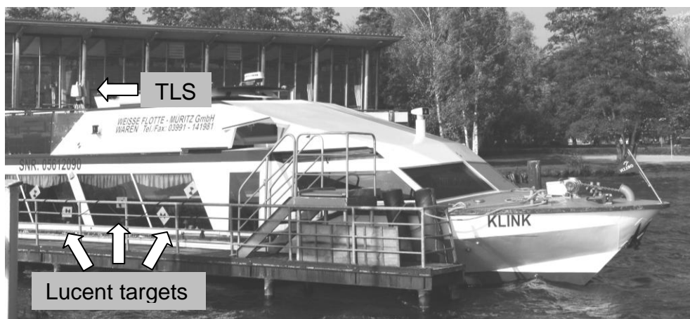
Figure 1: Front part of the Klink with lucent targets prepared for image acquisition
