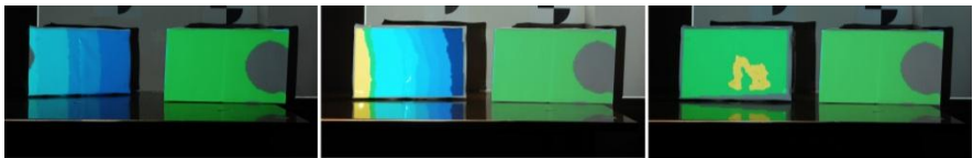
Figure 6: Processing steps of the alignment: initial position of the boxes (left), corrected location according to projected colour coding (middle) and final alignment (right).
