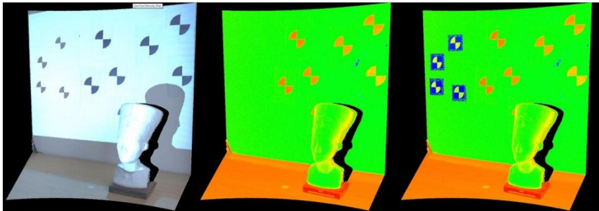
Figure 2: RGB image captured by the internal camera of the scanner (left), measured intensity information (middle), virtual targets derived from RGB imagery and physical targets (right)
