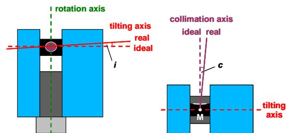
Figure 5: Tilting axis error and collimation error
