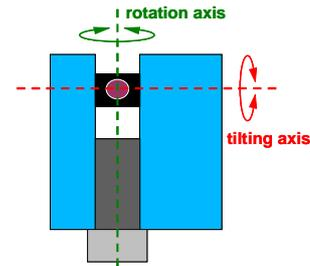
Figure 3: Rotation and tilting axes of Z + F Imager 5003
