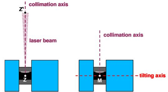
Figure 4: Collimation axis of Z + F Imager 5003
