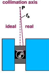
Figure 6: Eccentricity of the collimation axis
