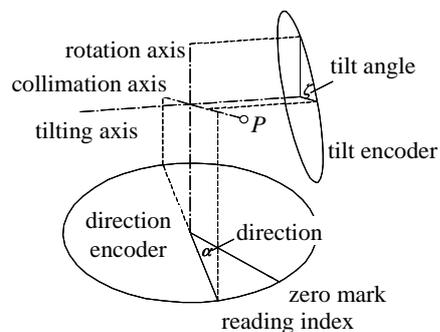
Figure 2: Axes and encoders of a polar measuring system
