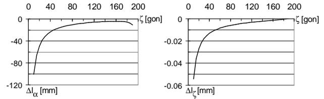
Figure 8: Position deviations  $\Delta l_\alpha$  and  $\Delta l_\zeta$  due to axes errors and eccentricity
